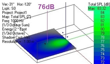
Figure VI. Placing one traditional loudspeaker we get 76dBspl.
