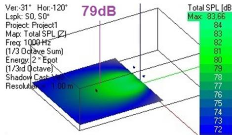
Figure VII. Placing two traditional loudspeakers we get 79dBspl.
